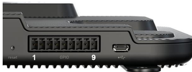
Figure 8: Impinj R700 Series GPIO Pin Locations
